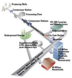
Figure 1: Typical pipeline delivery system.
